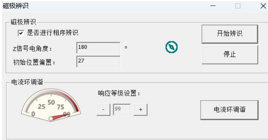
Figure 3-28 Magnetic pole identification
