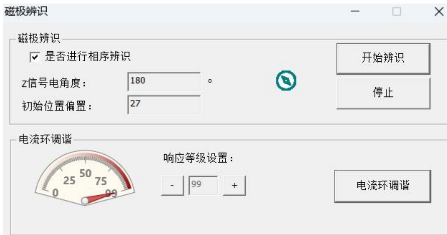
028Figure 3-28 Magnetic pole identification
