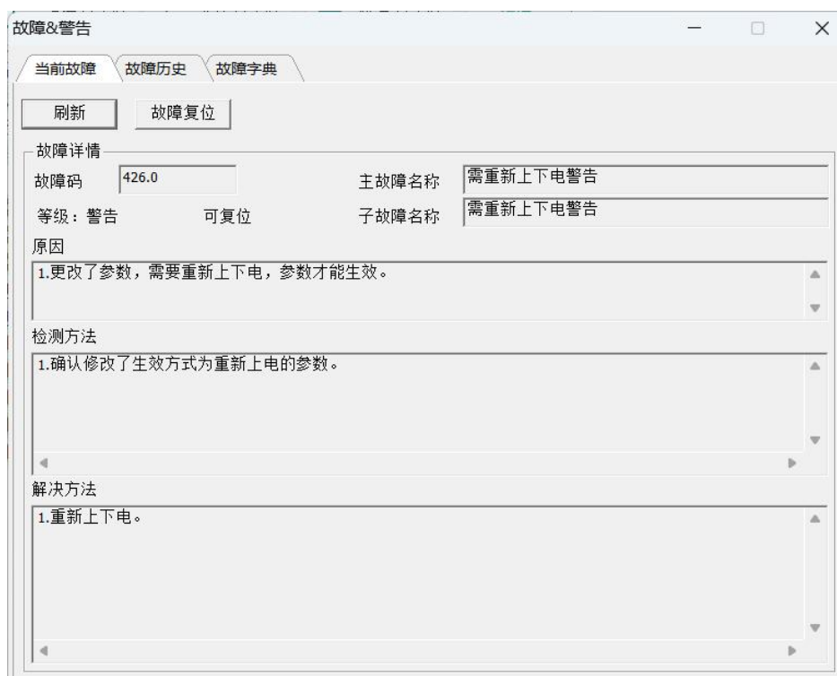
048Figure 3-48 Fault Diagnosis
